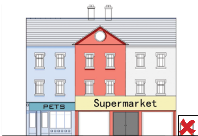
Lacks proportion and relationship with rest of building.
